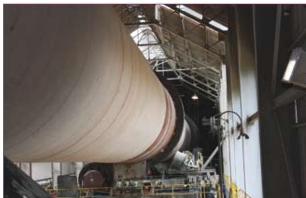
The company can provide 4 in. thick x 10 ft. wide x 50 ft. dia. kiln shell replacements.
