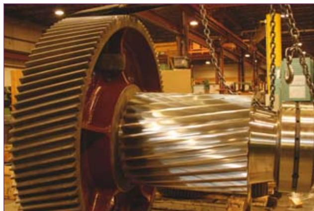
In this case, EuroGear quickly responded to recreate a pinion gear and reverse engineered it to fit into a different intermediate gear to save the client time and money.
